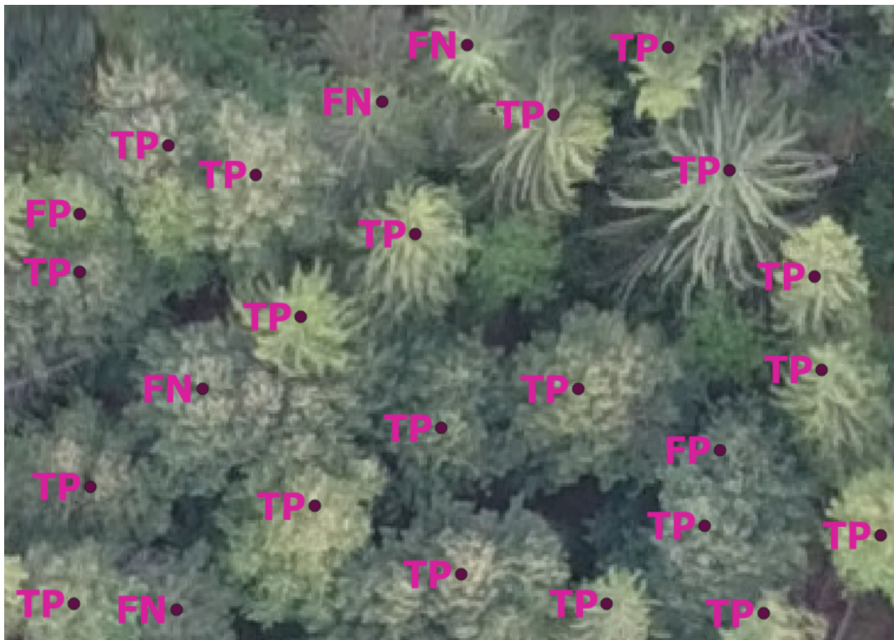
Fig. 3. Correctly detected trees (true positive = TP), false positives (FP), and trees missed by the algorithm (false negative = FN) on a fragment of an orthomosaic.
